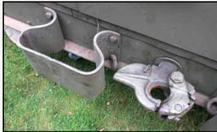
Kitpart A20 has to be rotated 90° when back door is opened.
