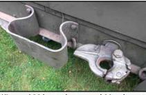
Kitpart A20 has to be rotated 90° when back door is opened.
