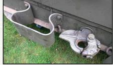
Kitpart A20 has to be rotated 90° when back door is opened.
