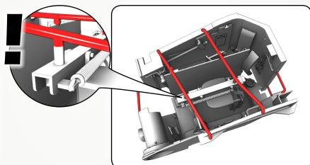
Please cut the red parts of, to remove parts from frame.
